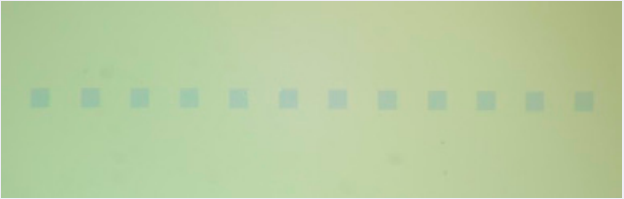
Figure 2: Graphene square flakes laser transferred directly on test substrates without any post-processing or patterning. Credit: National Technical University of Athens –Silex Microsystems
