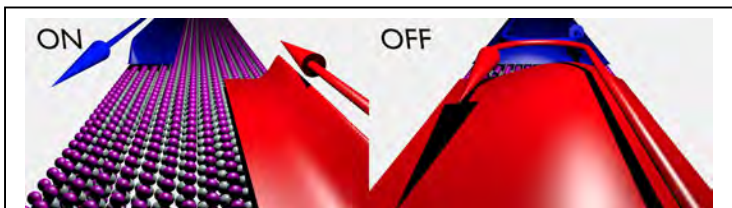
Fig. 1 Schematic operating principle a topological insulator-based FET in the on-state (left) and in the off-state (right).
