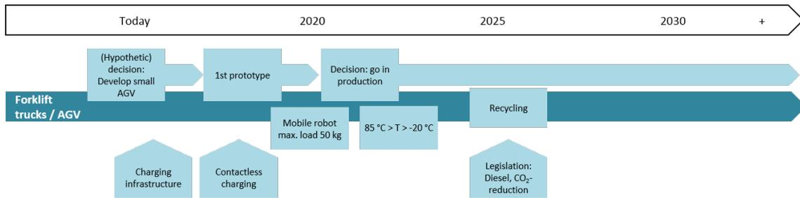
Figure 63: Roadmap for the development of an AGV.
