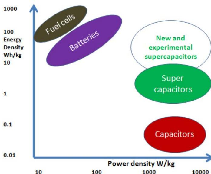
Figure 58: Energy density vs. power density for energy storage devices. [305]
