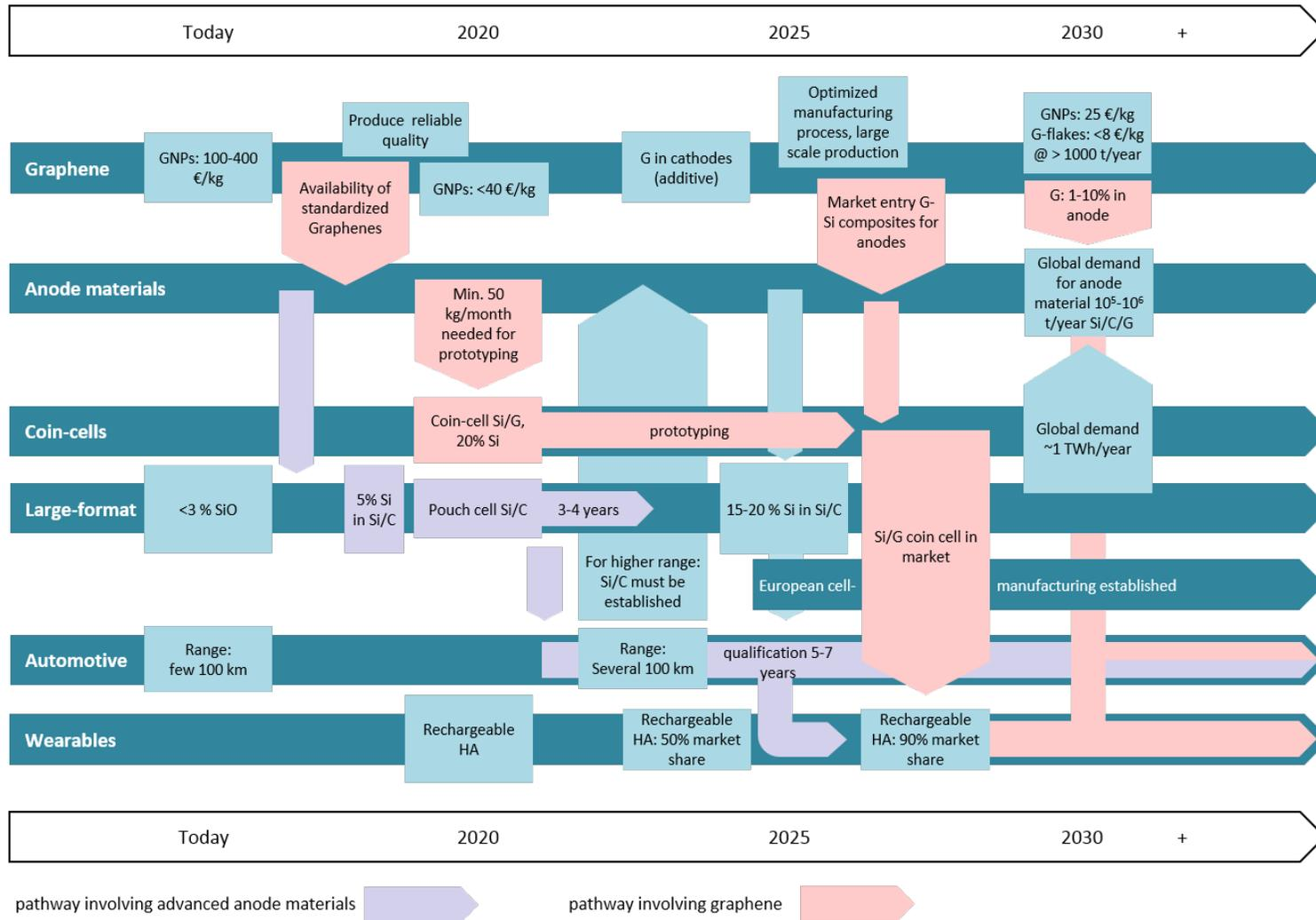
Figure 57: Interface roadmap for the introduction of graphene enhanced Si-anodes in LIBs for application in cars and wearables.
