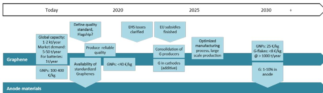
Figure 54: Roadmap for graphene-enhanced anode materials.
