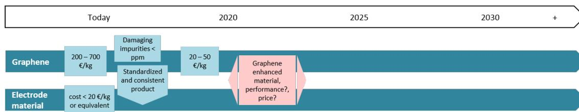
Figure 61: Roadmap for the further development of graphene-enhanced electrode materials for supercapacitors.
