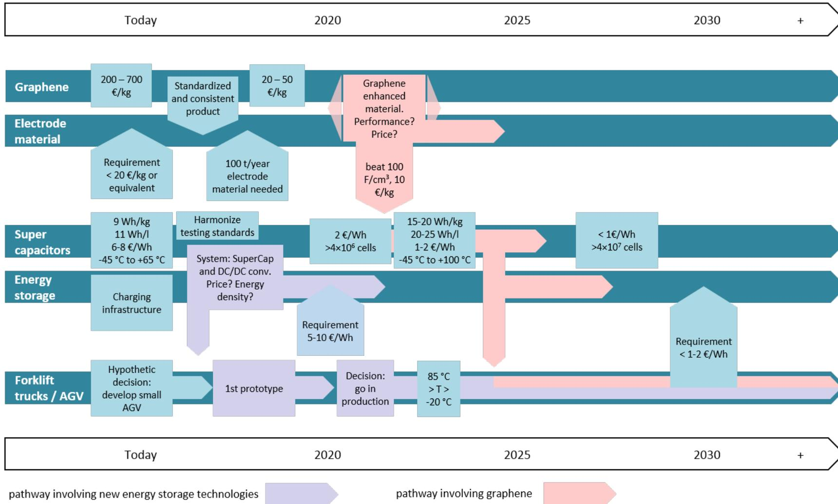
Figure 64: Interface roadmap for the implementation of graphene-enhanced materials in supercapacitors for forklift applications.
