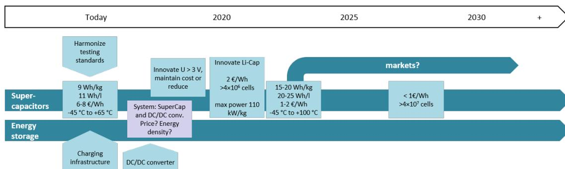
Figure 62: Roadmap for the further development of supercapacitors as storage devices in energy storage systems.
