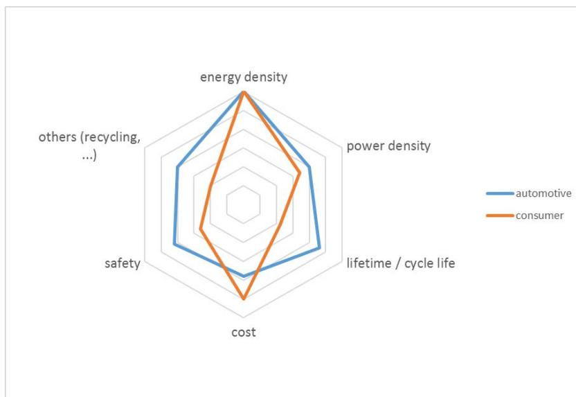
Figure 53: Generic spider diagram showing the requirements determined by different applications. A higher radius in the diagram means higher/stricter requirements
