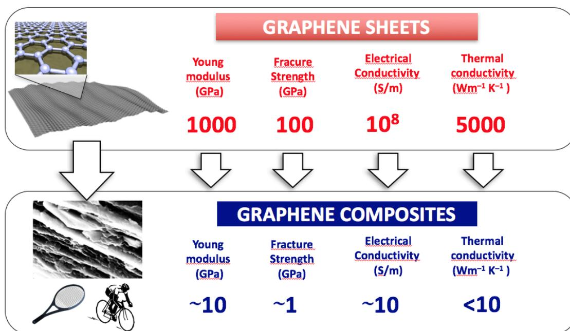
Figure 27: Properties of graphene sheets and current realisation in composites. [118–120]
