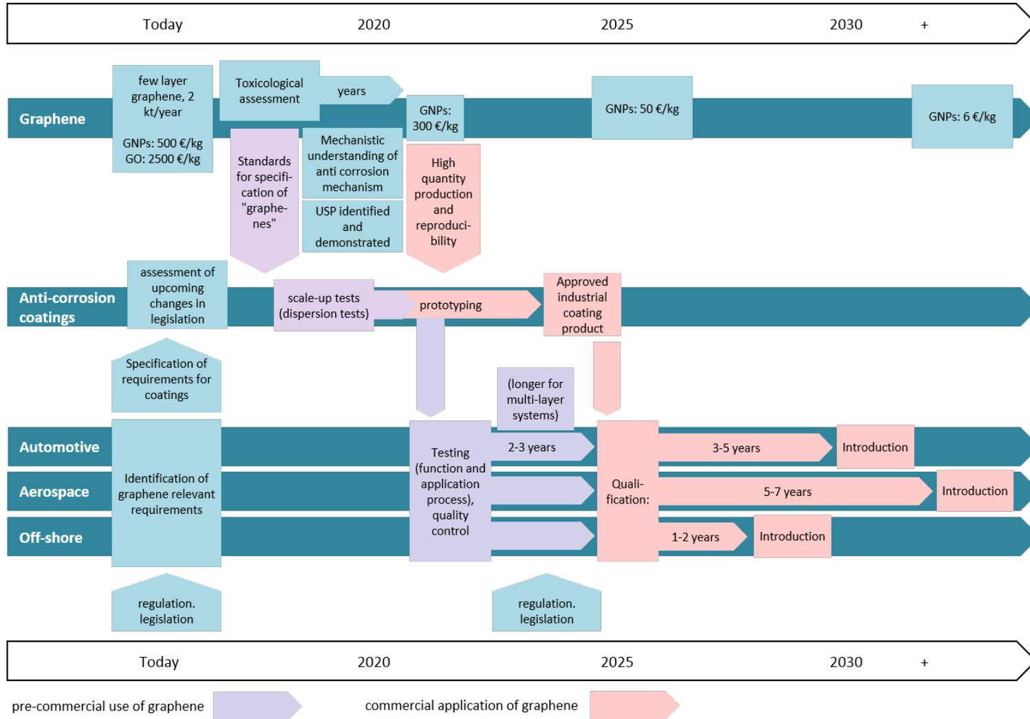
Figure 43: Interface roadmap for the introduction of graphene-based anti-corrosion coatings in automotive, aerospace and off-shore industries.
