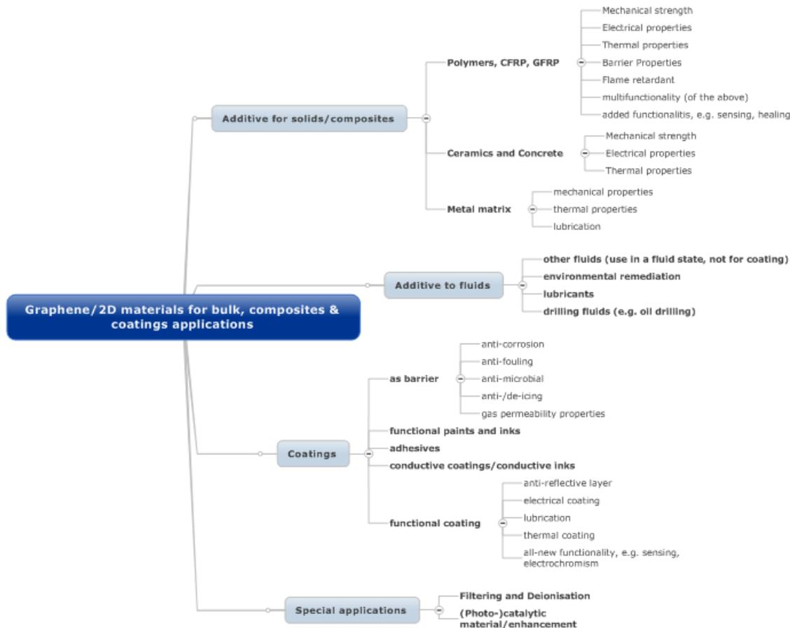
Figure 26: Potential applications of graphene and 2D materials covered in this chapter.
