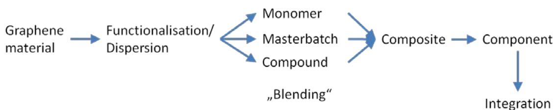
Figure 37: Simplified processing of polymer composites. The steps for other host materials are comparable with different processing techniques when it comes to composite preparation.
