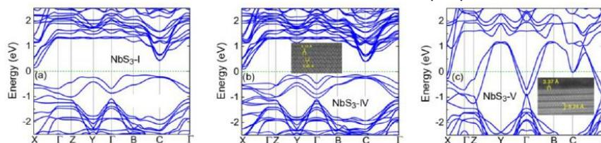
Fig. 1. Calculated energy momentum relations for NbS<sub>3</sub> phases I (a), IV (b) and V (c). TEM images are inset in (b) and (c) that show the atomic distances [3]. The dimerization is apparent in NbS<sub>3</sub>-IV.
