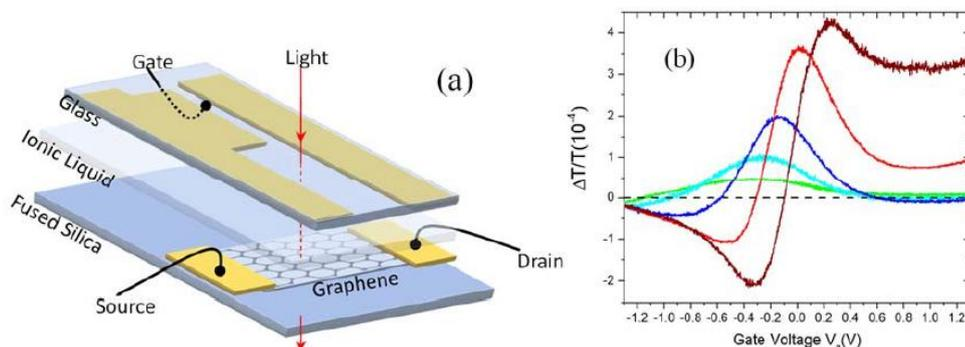
Figure 1: (a) scheme of the SLG device gated with ionic liquid; (b)  $\Delta T/T$  dynamics at zero pump-probe delay following excitation at  $\omega_{pu} = 0.8$  eV, for probe photon energies  $\omega_{pr} = 0.75$  eV (brown), 0.88 eV (red), 1 eV (blue), 1.13 eV (light blue) and 1.24 eV (green).
