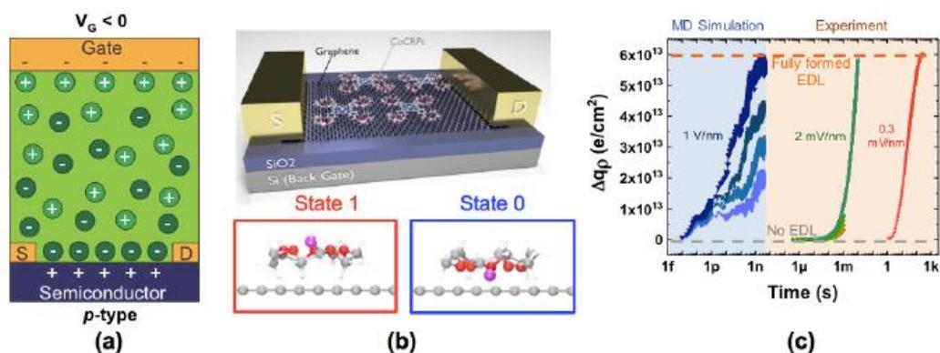
Figure 1: (a) Schematic of electric double layer (EDL)-gated FET. Negative topgate bias ( $V_G$ ) drives anions to the surface of the semiconductor inducing p-type doping. (b) Schematic of monolayer electrolyte doping a graphene FET, and the two possible states. (c) Sheet density versus time showing the time-dependence of EDL formation in response to three different electric field strengths: 1
