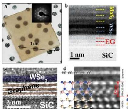
Fig.1: Examples of (a) wafer-scale WSe<sub>2</sub>, (b,c) 2D heterostructures, and (d) 2D-Gallium Nitride.
