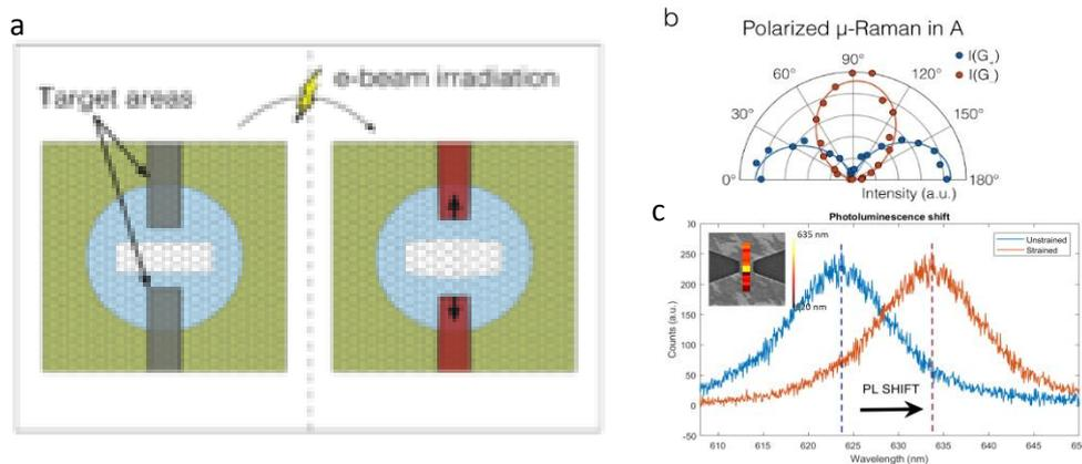
Fig. 1. (a) Example of device architecture involving two MAMs. Uniaxial strain in the central region is expected. (b) Local uniaxial stretching induced on graphene using two MAMs and demonstrated with polarized micro-Raman spectroscopy. (c) Photoluminescence spectrum and map (inset) of WS<sub>2</sub> uniaxially strained in between two MAMs.
