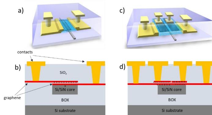
Figure. 3D image and cross section of a) – b) graphene double layer modulator on silicon waveguide and, c) – d) split gate photodetector based on photothermal effect
