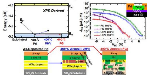
Fig. 1. Impact of post-metal anneals on Fermi level control, transport and the associated interfaces for Pd/WSe<sub>2</sub> ohmic hole contacts. After [11].
