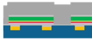
Sealing and cladding of 2D active patches to avoid delamination (existing infr.)
