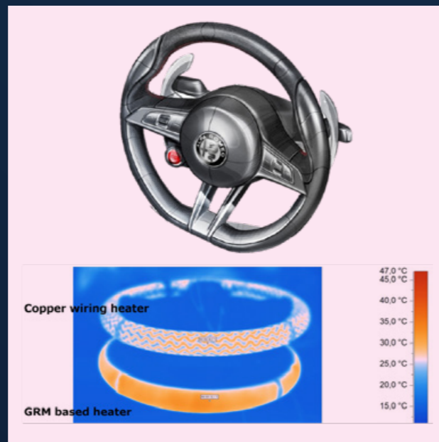
A G+BOARD steering wheel demonstrator with integrated heating capabilities showing the differences between traditional copper wiring and a GRM-based approach. Credit: Stellantis
