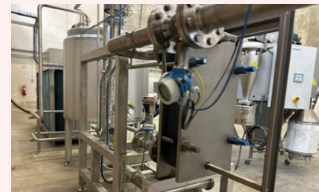
Installation of Graphenest's solvent recovery system, enabling cleaner and more efficient production of graphene-based EMI shielding materials. Credit: Graphenest
