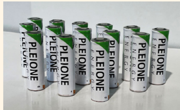
Graphene-based Lithium-ion cylindrical battery cells and battery module assembly integrating multiple lithium-ion cells for space applications. Credit: Pleione Energy GmbH
