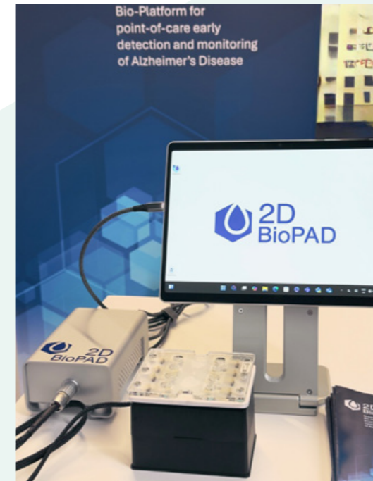
Figure 1. 2D-BioPAD GFET-based prototype biosensing platform. Credit: 2D-BioPAD
