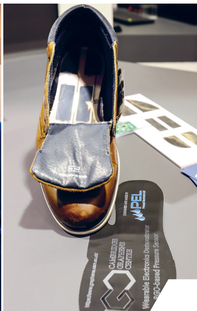
Pressure sensing insoles made of lightweight graphene-embedded foam could be integrated into any type of shoe.
