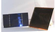
*Figure 1: comparison between silicon solar cell (left) and graphene-perovskite solar module (right)*
