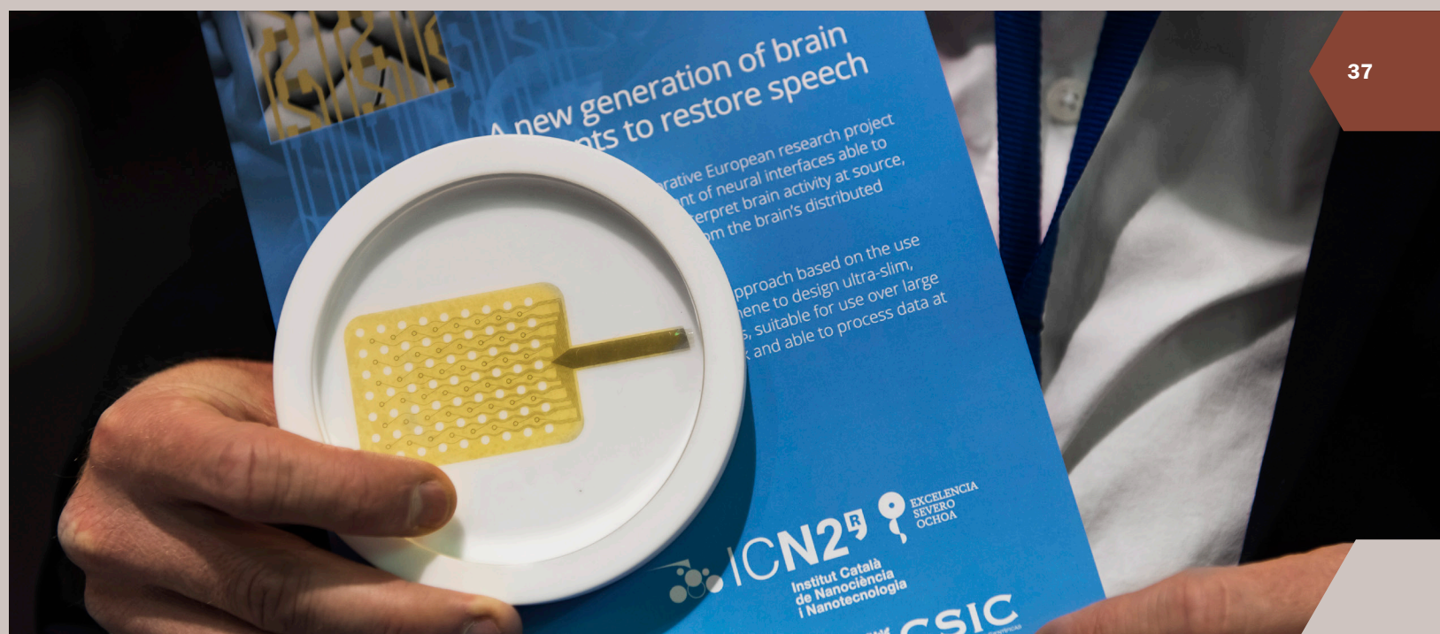
Flexible arrays of graphene solution-gated field effect transistors can be used to monitor brain activity. Credit: Alexandra Csuport
