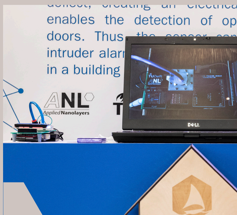
A battery-powered capacitive pressure sensor consisting of 10,000 membranes. Credit: Alexandra Csuport
