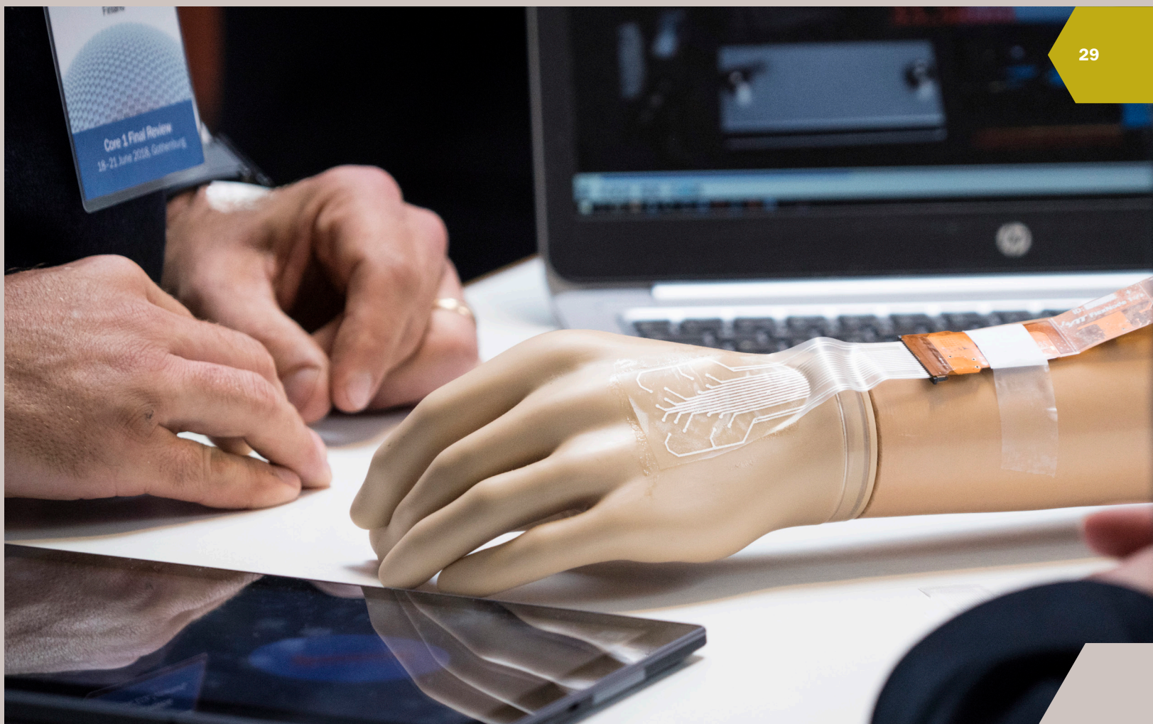
This wearable epidermal sensor grid can be used as the basis for a wide variety of wearable autonomous devices. Credit: Johan Bodell/Chalmers
