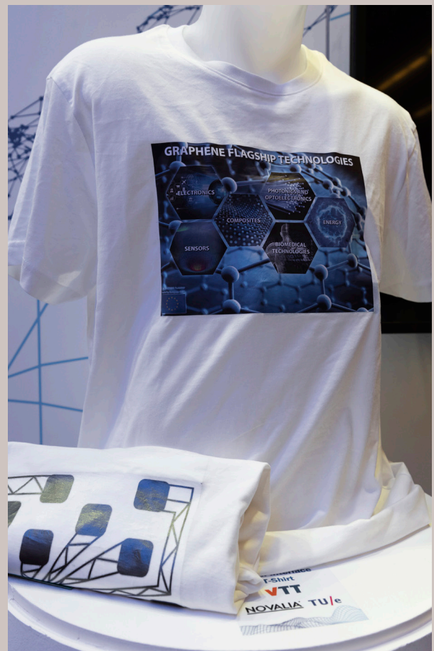
Graphene is well suited to printing conductive tracks and areas onto flexible surfaces, such as plastic sheets, paper or fabrics. This shirt integrates graphene-based, electrically conductive areas that function as capacitive touch sensitive electrodes. Credit: Alexandra Csuoport
