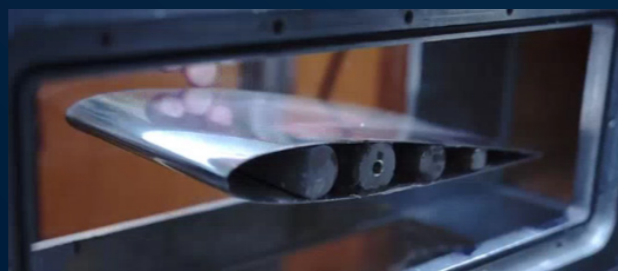
A small-scale demonstrator was subjected to tests in the Airbus iCORE Icing Wind Tunnel to assess the performance of GRM technologies for de-icing applications. Credit: Airbus
