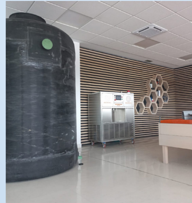
A non-metal chemical reactor for potentially explosive atmospheres, based on graphene composites to gain electrical conductivity, fire retardancy and anticorrosion properties. Credit: Julio Gómez-Cordón, Avanzare
